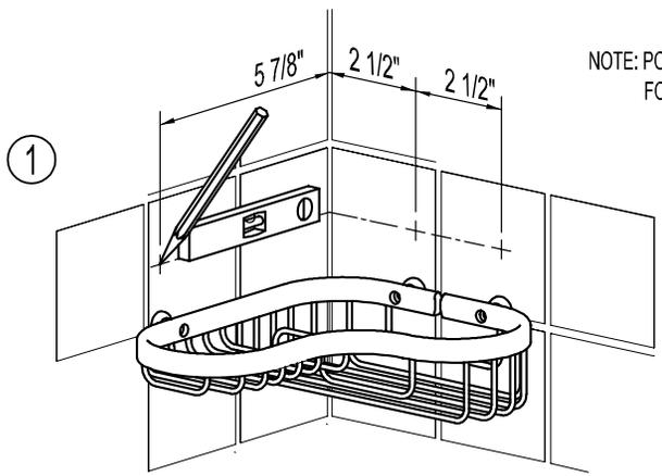
NOTE: POST MUST BE USED FOR MARKING HOLES
